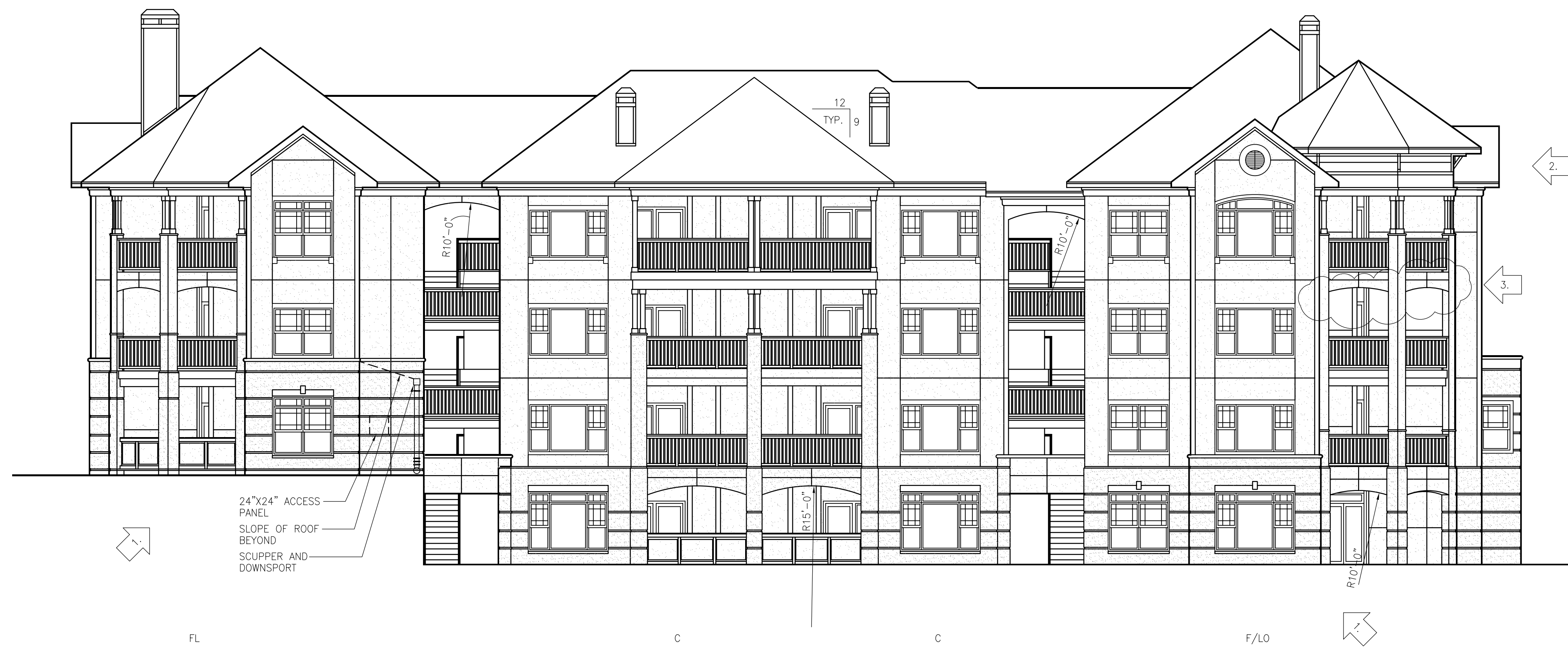
ELEV. 1 BLDG 100 1/8"=1'-0" A3.1 REAR ELEVATION WEST
